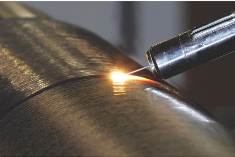
Wire as the filler material can be advantageous, especially for cylindrical part geometries. Wire feed can also be made into a hybrid process with the integration of a hot wire power supply for pre-heating the wire while being fed into the molten puddle.
