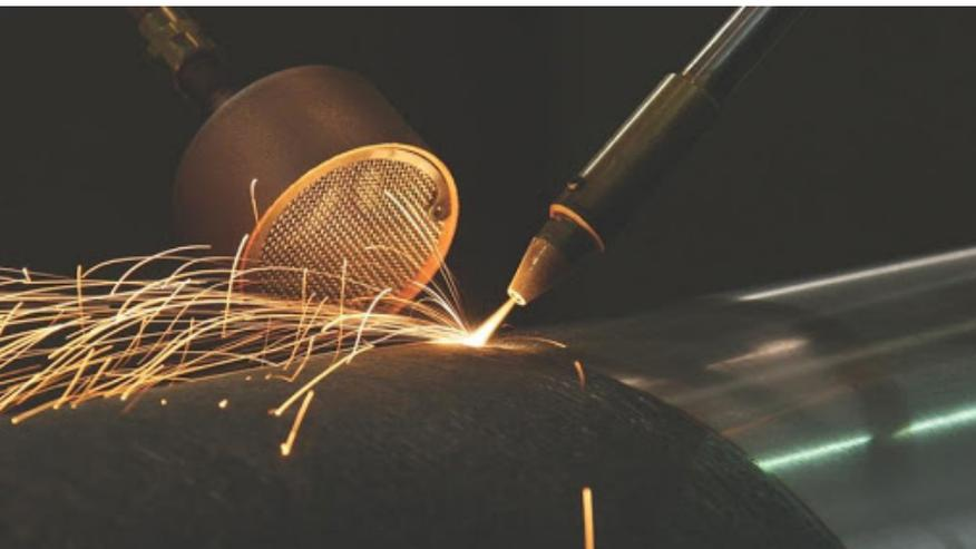
Laser cladding with coaxially configured powder nozzles enables multi-axis motion systems where the head is steered to follow the contours; for example, cladding for part repair. Worn edges of the part can be built back up and then machined to finish dimensions.
