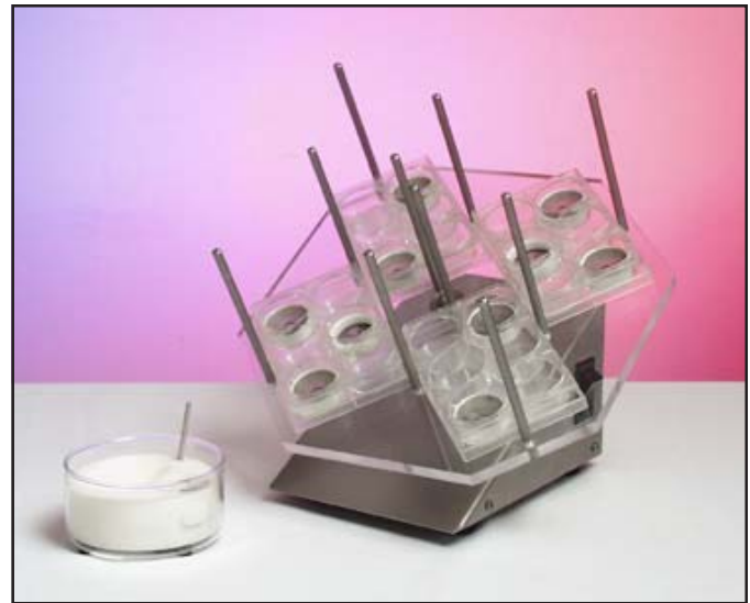
Incubation unit with well plate holders, well plate inserts, and tissue slicer loader.
