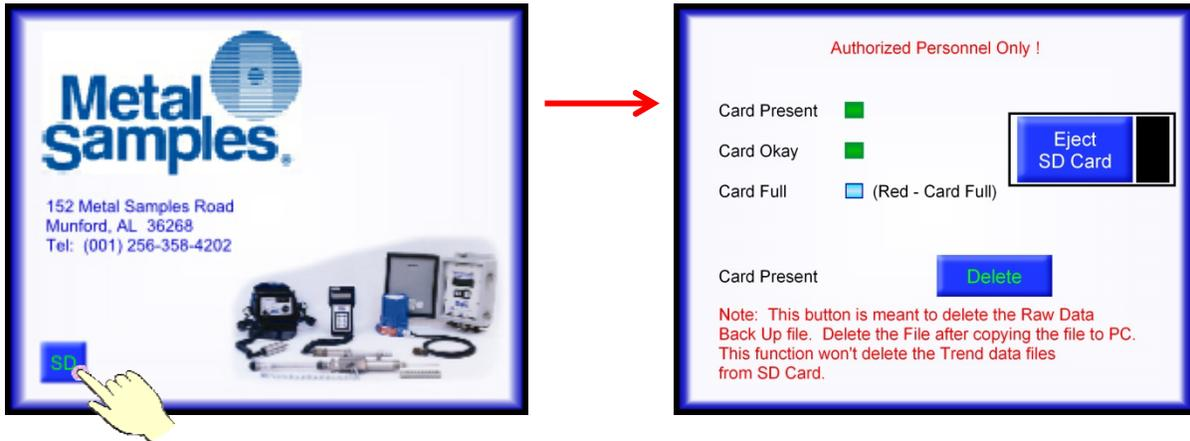
The SD management screen gives several status messages about the microSD memory card and has a button to delete the raw data backup file. Use this function when a card is full to easily clear space.
