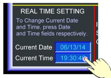
This will open the numeric keypad and allow the new date or time to be entered. Press the return key **↵** when finished to accept and enter your changes, or press the escape (ESC) key to abort your changes.
