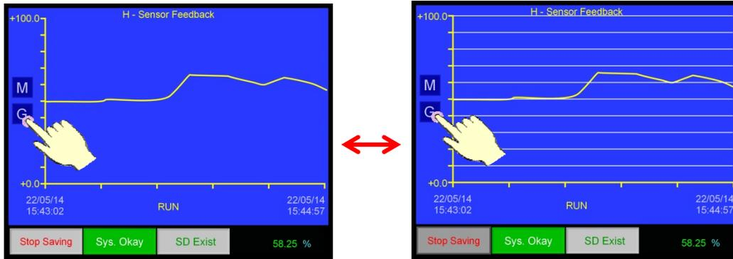
**Manual scroll** – Pressing the ‘M’ button on the left side of the screen will bring up the manual scroll buttons, allowing you to scroll back and forth through the recent data history. When you are done, press the ‘M’ button again to hide the manual scroll buttons and return to “Run” mode.
