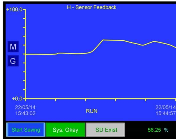
**MicroSD Card Status** – The MS3112 checks to make sure a microSD card is present for data storage. The SD status message box along the bottom of the main display will indicate “SD Exist” when a microSD card is present, or “SD not Exist” when one is not.
