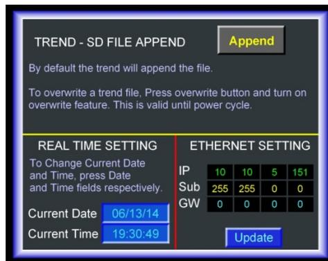
**TREND – SD FILE APPEND (Save Mode)** – By default the MS3112 recorder will append new data to the existing file if you stop and restart data saving. If you prefer for new data to overwrite the old data, press the Overwrite button to change from Append to Overwrite mode.
