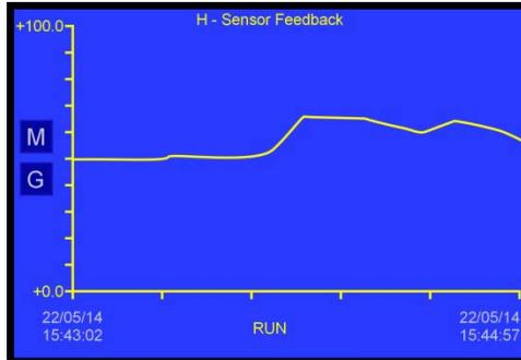
It is important to note that the vertical scale of the graph is *percentage*. The actual magnitude of the vertical scale depends on the setting of the Current range switch. For example, if the Current range switch is set to 200  $\mu\text{A}$ , then the vertical scale of the graph is equivalent to 0 to 200  $\mu\text{A}$ .
