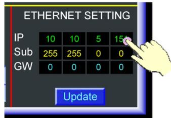
To change any of these values touch the desired box. This will open the numeric keypad and allow the new values to be entered. Press the return key **↵** when finished to accept your changes, or press the escape (ESC) key to abort your changes.
