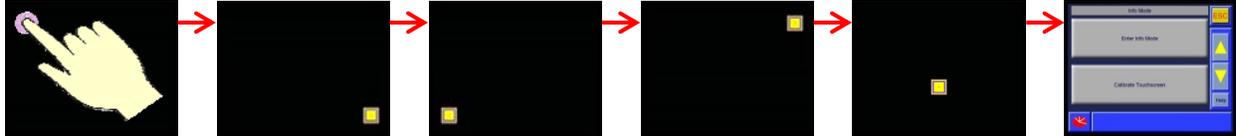
After touching the calibration mark it will move to a new position on the screen. Touch it again each time it moves until the instrument returns to the “Info Mode” screen. At this point the touchscreen calibration is complete, and the positional accuracy should be more precise.
