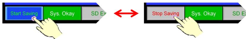
*\*NOTE: On some occasions the button may display “Stop Saving” immediately upon startup, indicating that the unit is already logging data. If this happens, an error has occurred and the unit is giving a false indication. In this case press “Stop Saving” then press “Start Saving” to ensure that the unit begins logging data.*
