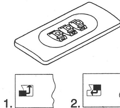
The combination of the lock on the MS3112 case is factory set at 0-0-0.
