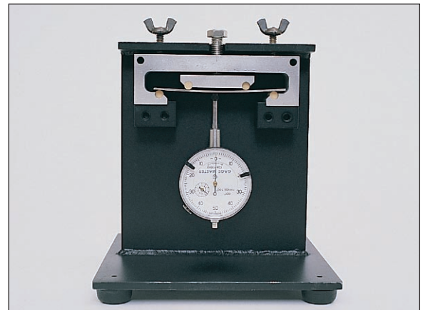
P/N TF2404 Stressing Frame For use with P/N TF2445
