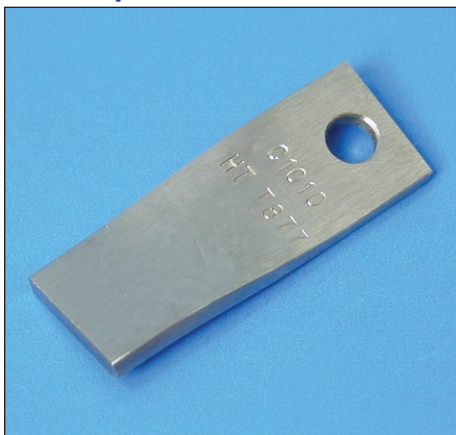
P/N CO303 Twist Specimen
