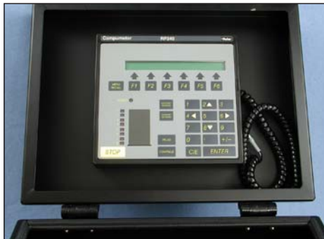
The control panel fits on the lid of the enclosure.
