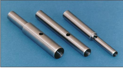
Our new improved coring tools are used for cutting cylindrical live tissue cores for use in the Alabama R&D Tissue Slicer. Thin wall stainless steel tubing used in other coring tools does not hold an edge well and is difficult to sharpen. The new coring tools are made from heat-treated, knife-quality stainless steel. The cutting edge angles are designed to give sharp, well-formed tissue cores which is important for use in the Alabama R&D Tissue Slicer.
