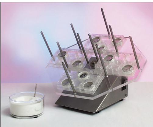
Alabama R&D's Incubation Unit has been designed to provide optimal oxygenation and nutrient delivery to tissue slices in organ culture and to minimize damage and facilitate handling of the slices during preparation.
