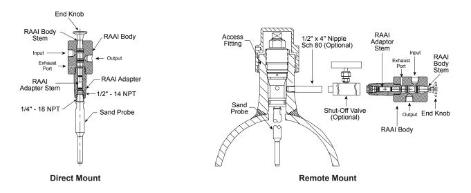
**Model PR6573158** is a remote alarm actuator / indicator (RAAI) which can be used with a sand probe to indicate when erosion penetrates the probe. The RAAI may be mounted directly on the probe or may be mounted remotely to a tee type access fitting body which is connected to the probe.
