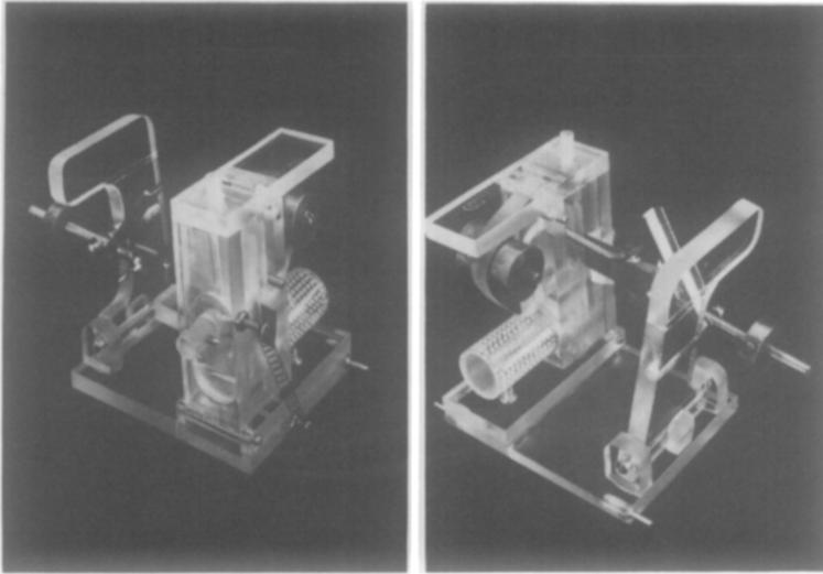
FIG. 1. Front and rear view of the microtome.
