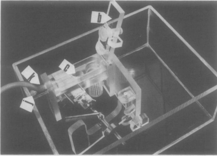
FIG. 3. Microtome in "load" position inside box for isotonic medium: See (b), spring-loaded door; (c) sample well.
