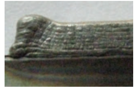
Fig. 7 — Multipass laser metal deposition with precision wire feeder.
