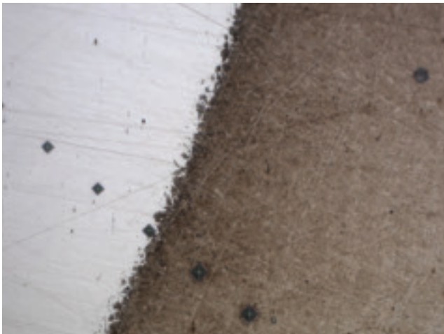
Fig. 1 — Laser clad deposit of 420 stainless steel on 4140 (200×).
