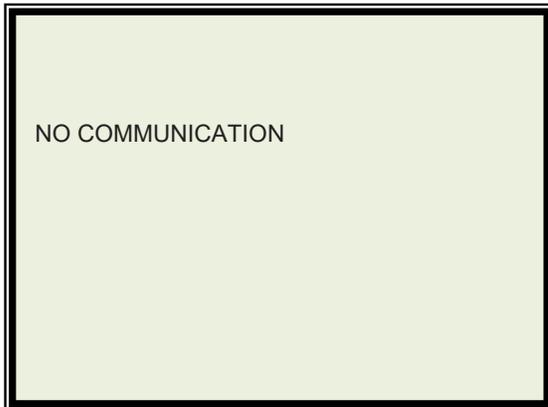
If this error occurs, ensure that all of the current loop cable is connected. Ensure that you are using the Metal Samples current loop cable that was shipped with the data logger.
