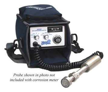
since it can be used in conductive and nonconductive environments, such as petroleum, chemical, water, soil, or even atmosphere.
