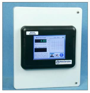
The MS2540 also offers an integrated web server. This feature allows users to access the MS2540 from any PC on the network using a standard web browser. Through this interface users can view data and make setup changes to the MS2540.
