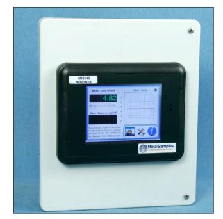
The MS2540 also offers an integrated web server. This feature allows users to access the MS2540 from any PC on the network using a standard web browser. Through this interface users can view data and make setup changes to the MS2540.
