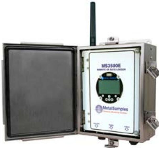
The MS3500E takes probe readings on a user-programmable logging interval. Readings are time and date stamped as they are taken, then stored to memory. Between readings, the instrument remains in a “sleep” mode to conserve main battery power. The instrument’s memory is capable of storing more than 100,000 readings, and is stored in non-volatile Flash memory.
