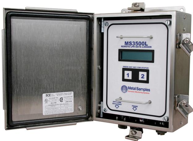
The MS3500L incorporates a high-precision zero-resistance ammeter (ZRA) for measuring galvanic current between electrodes. It also offers a high-precision voltmeter for measuring the open-circuit potential between electrodes.
