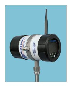
The MS5000E-ISA takes probe readings on a user-programmable interval. Readings are then transmitted wirelessly using the ISA 100 protocol. Between readings, the instrument remains in a "sleep" mode to conserve main battery power. It is supplied with a Lithium battery pack which has a standard life of 3 years under normal working conditions and is certified to be replaced in hazardous locations.
