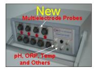
**Model S-50:** Measures real-time corrosion rates, corrosion potentials, temperature and other parameters simultaneously from four independent Coupled Multielectrode probes, three pH or three ORP probes, or three other transducers for parameters such as conductivity, humidity, flow, and pressure.
