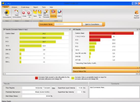
Figure 2: Predict ® -Crude 2.0 program output interface, showing corrosion predictions
