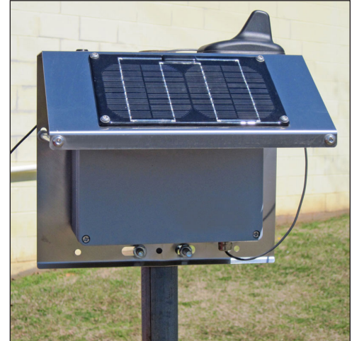
Remote corrosion monitoring telemetry system with solar panel
