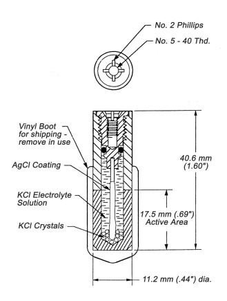
When removing the TF0221 electrode from the probe, it is important that both the electrode body and the Viton® gasket be grasped, then turn both counter-clockwise. If the electrode is removed by turning the electrode body only, then the silver internal element may be unscrewed from the electrode casing.
